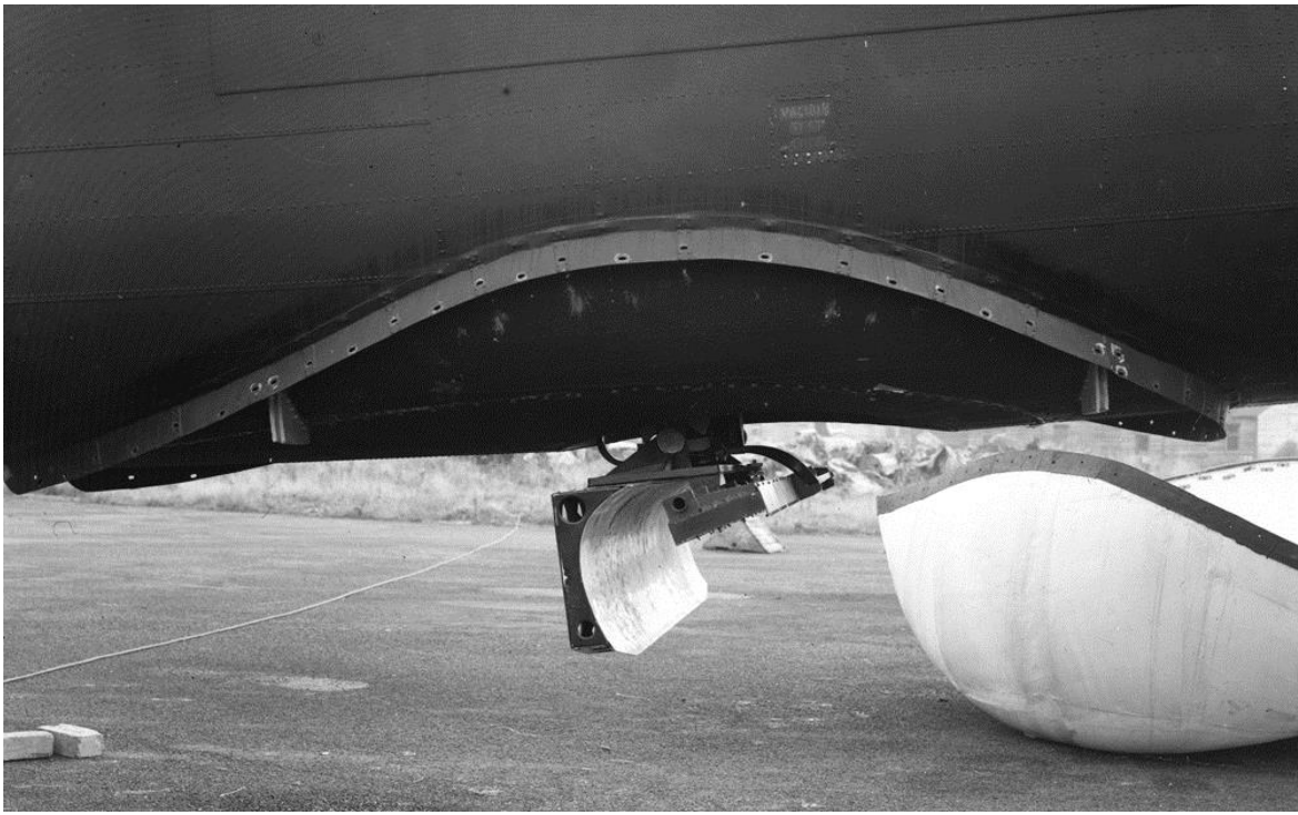
H2S Mk IVA scanner on the underside of Lincoln RE229.
