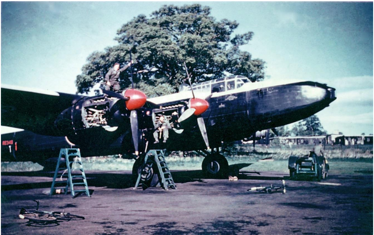
The nose of Lincoln RE346 was modified in 1953 for infrared trials, though the ventral H2S radome was retained. This is the only known colour photograph of an aircraft at Defford. (H Badger)
