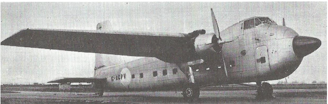
ABOVE: Wayfarer VR380 featuring the radar scanner on the nose. VR380 reverted to civilian status as G-AGPV in 1958 but at the date of this photo, it still displayed the nose radome (more on the radar installation in VR380 on the next pages.
