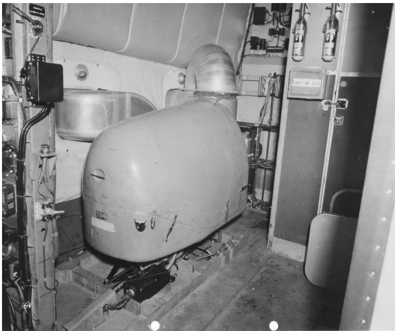
ABOVE: interior of VR382 taken July 1954 showing Rotol APU (Auxiliary Power Unit)
