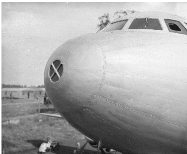
LEFT: VX199 fitted with an infrared detector system in its nose
